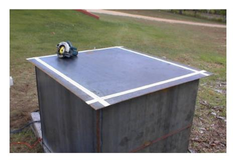
Orient the firebox so the front is skyward. Mark the fire door opening on the face of the front. The mark should be 1/2" inward on each side so a welding flange will be available after the door opening is cut. The author originally planned to use 2" wide masking tape to facilitate the marking but found a black magic marker to work the best.
