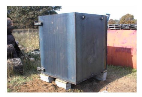
The author used solid 8" wide x 16" long by 4" thick solid concrete blocks on solid, undisturbed ground along with varying thickness' of plywood and shim material. The stove should be level and solidly supported around the entire perimeter.
